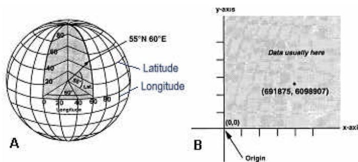
**Figure 3.9** Spherical and Cartesian Coordinate Systems.
